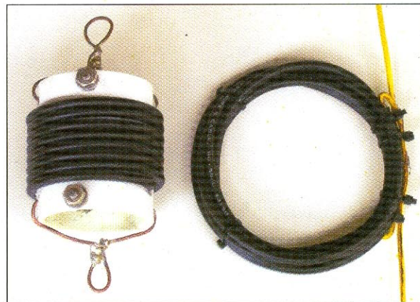
Figure 2 — Common PVC form trap compared to the 40 meter version described in this article.
