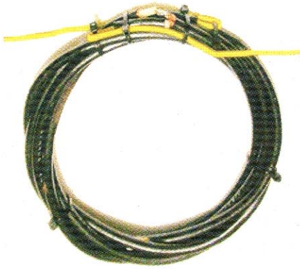
Figure 7 — A no-form coax antenna trap No-form traps have four very real advantages: They are easy to make with a whole number of turns, they are lighter in weight, lower in cost and simpler to fabricate.
