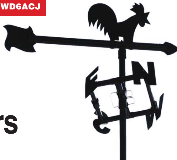
Figure 1—The completed weather vane antenna. Can you find the loop?
