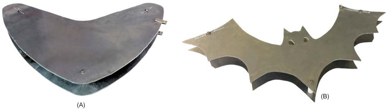
Figure 4 — Alternative shapes are also possible. At (A), a boomerang shape is aesthetically more pleasing than the square, but requires more fabrication effort. At (B), the novelty bat-shaped antenna is always a fun attention-getter.
