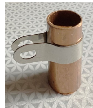
Figure 10: Re-shaped stainless cable clamps for ends of adjustment bars.
