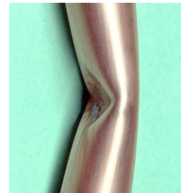
Figure 6: Bend at half flattened spot in pipe
